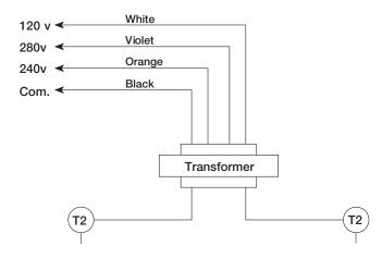
Model M4182 Wiring Connections Note: Model M8182 is a 24 Volt actuator with no transformer. Connections must be made directly to T1 and T2.
